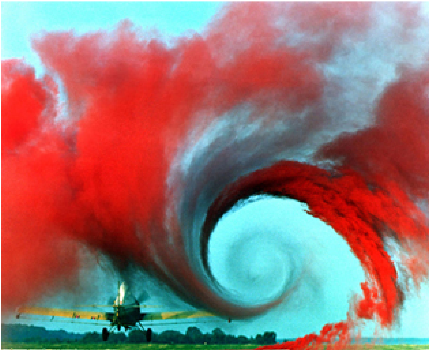
Figure 5: This image shows a trailing vortex from an aircraft wing, visualised by red smoke.
