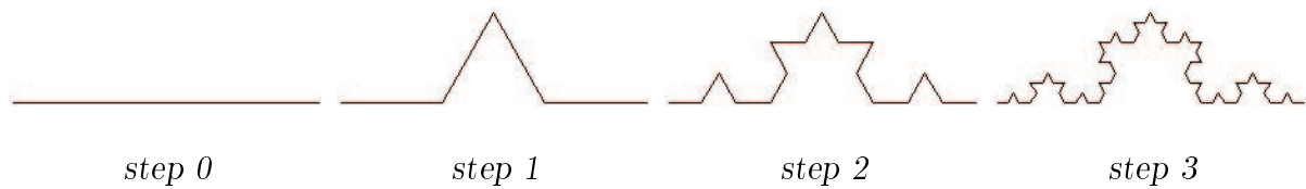
Figure 8. Construction of the Von Koch curve. One starts with a simple line segment. Then, at every stage of the iteration, one cuts each line segment into three, and replaces the middle piece by two new connected segments (sticking outward), each of the same size as the two remaining original pieces. This is repeated an infinite number of times.
